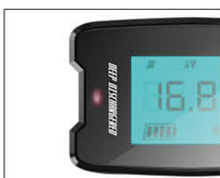
Low voltage indicator: Red LED
